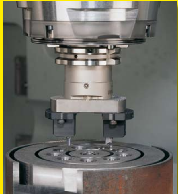
Face grooving with URMA IntraMax and boring with URMA fine boring head
