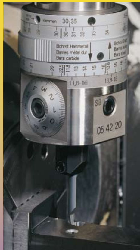
Face grooving with URMA IntraMax and boring with URMA fine boring head
